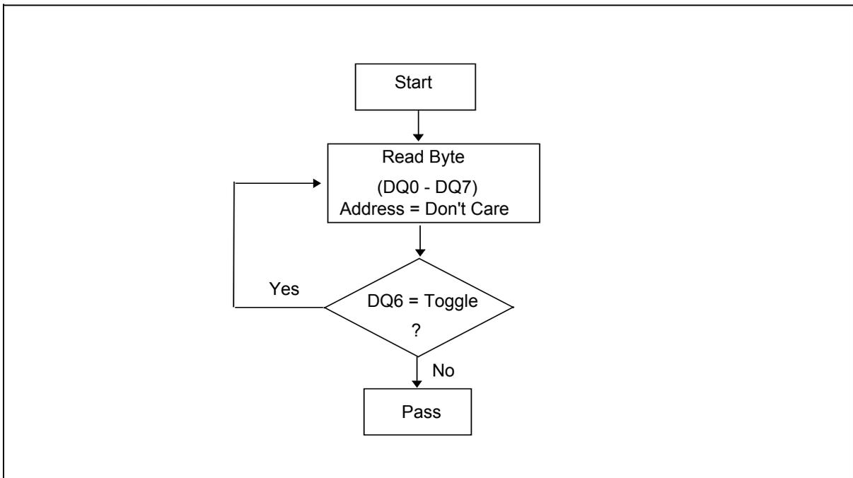
**Boot Block Lockout Enable Flow Chart**
