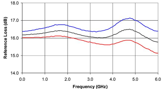
Attenuation - 16 dB Bit (C2) vs. Frequency
