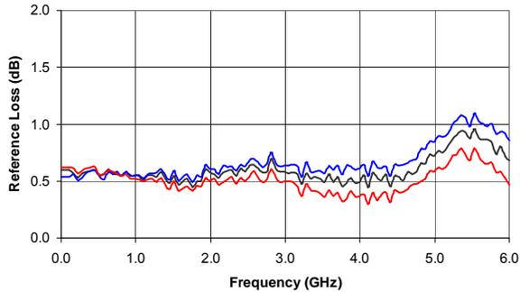
Attenuation - 16 dB bit (C1) Bit vs. Frequency
