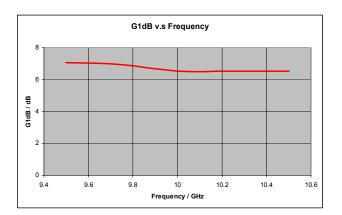
$V_{DS} = 10 \text{ V}, I_{DSQ} \approx 5000 \text{mA}$
