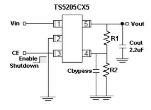
CE (pin 3) may be connected directly to Vin (pin 1) Low noise operation: Cbypass=470pF, Cout>2.2uF Basic operation: Cbypass=not used, Cout>1uF
