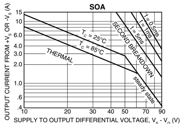
1. Capacitive and dynamic\* inductive loads up to the following maximum are safe with the current limits set as specified.
