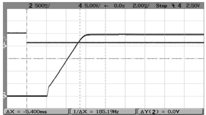
On/Off Enable Startup (VIN=5V, V out =2.5V, I out =6A, Cload=0) Trace 4=Enable, Trace 2=V out
