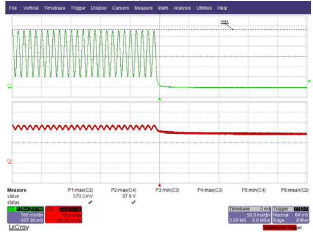
Figure 42 – 265 VAC 50 Hz, Output Fall. Upper: I_{OUT} , 100 mA / div. Lower: V_{OUT} , 10 V, 500 ms / div.
