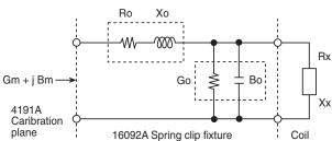
$\begin{array}{lll} \text{Gm + jBm:} & \text{Measured admittance [S]} \\ \text{Ro + jXo:} & \text{Residual impedance } [\Omega] \\ \text{Go + jBo:} & \text{Stray admittance [S]} \\ \text{Rx + jXx:} & \text{Unknown impedance } [Q] \\ \end{array}$
