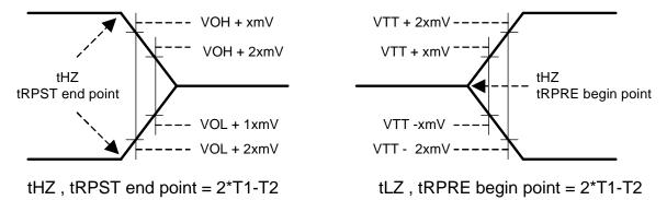
20. Input waveform timing with differential data strobe enabled MR[bit10] =0, is referenced from the input signal crossing at the  $V_{IH}(ac)$  level to the differential data strobe crosspoint for a rising signal, and from the input signal crossing at the  $V_{IL}(ac)$  level to the differential data strobe crosspoint for a falling signal applied to the device under test.
