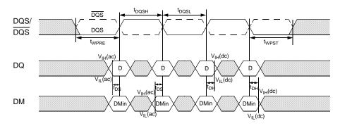
Figure -- Data input (write) timing
