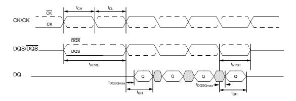
Figure -- Data output (read) timing
