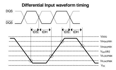
22. Input waveform timing is referenced from the input signal crossing at the  $V_{IH}(ac)$  level for a rising signal and  $V_{IL}(ac)$  for a falling signal applied to the device under test.
