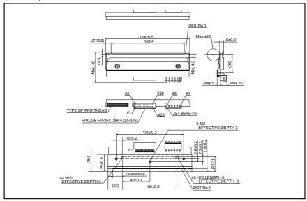
Note: No heat history control function inside the thermal printhead. External heat history control is required for high speed printing
