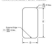
Note: The external edges (installation side) on the "D" sides of the cutout should have a minimum .020" radius. For optional retention against extraction, the corresponding inner edge should be sharp, without paint or coatings. Edge coatings, including anodization are also discouraged for good shield contact.
