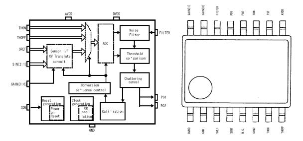
Sensor I/F CV Conversion Circuit:
