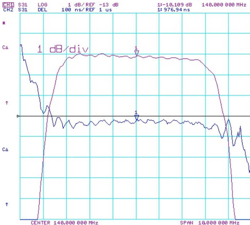
Fig2.S21 Response Horizontal:1MHz/Div Vertical: 1dB/Div
