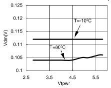
Differential Mode Bias Vdm vs. Temperature@Vtpwr=5V
