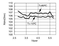
Differential Mode Termination Resistance Rdm vs. Temperature
