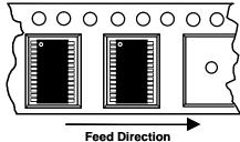
Typical SSOP, TSSOP Package Orientation
