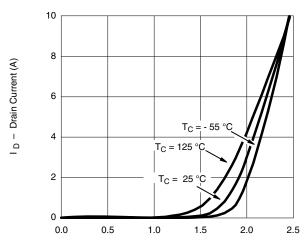
V<sub>GS</sub> - Gate-to-Source Voltage (V) **Transfer Characteristics**
