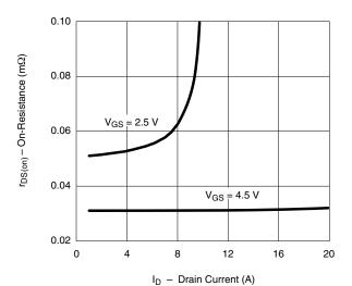
On-Resistance vs. Drain Current and Gate Voltage
