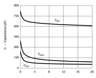
V<sub>DS</sub> - Drain-to-Source Voltage (V) **Capacitance**
