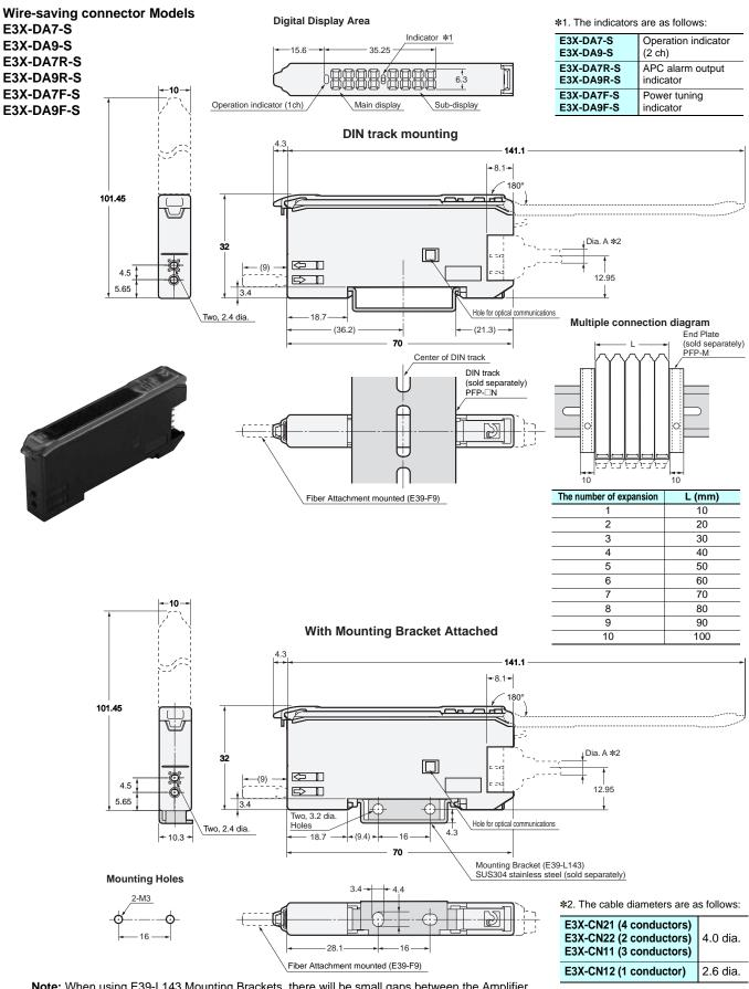
**Note:** When using E39-L143 Mounting Brackets, there will be small gaps between the Amplifier Units if they are mounted side by side.
