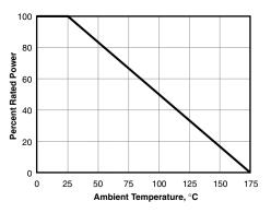
Derating (thermal resistance): 0.666W/°K (1.5K/W). Without a heatsink, when in free air at 25°C, the TEH100 is rated for 3.5W. Derating for temp. above 25°C is 0.0234W/°K.
