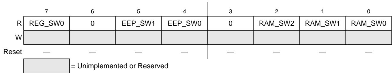
Figure 19-9. Memory Size Register 0 (MEMSIZ0)
