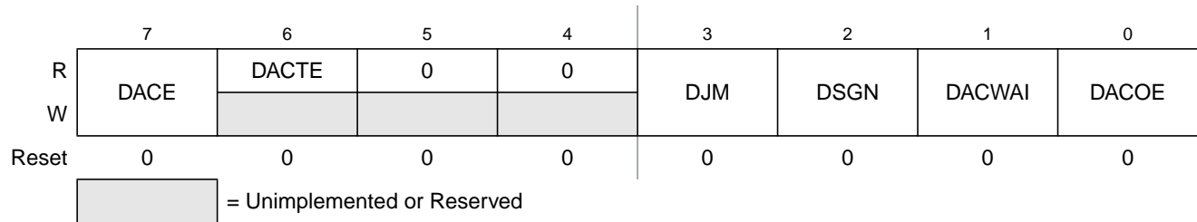
Figure 7-3. DAC Control Register 0 (DACC0)
