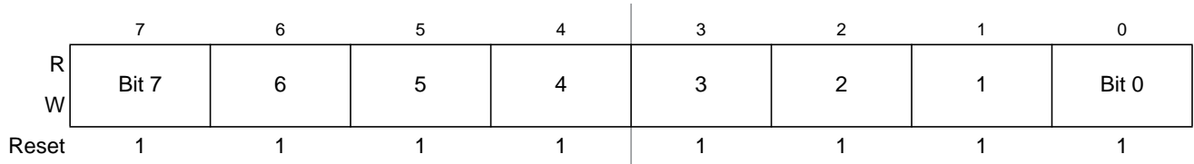
Figure 12-27. PWM Channel Duty Registers (PWMDTY0)
