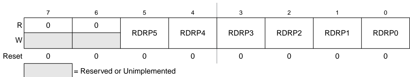
Figure 3-20. Port P Reduced Drive Register (RDRP)
