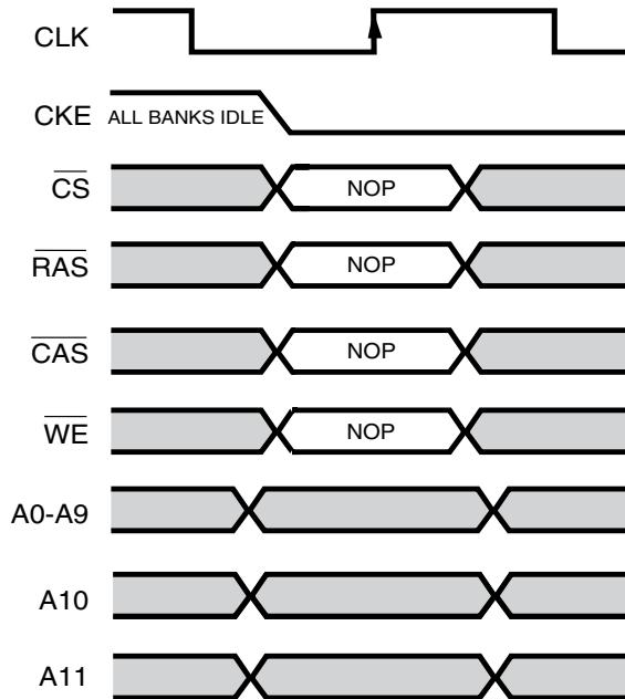
**Clock Suspend Command**
