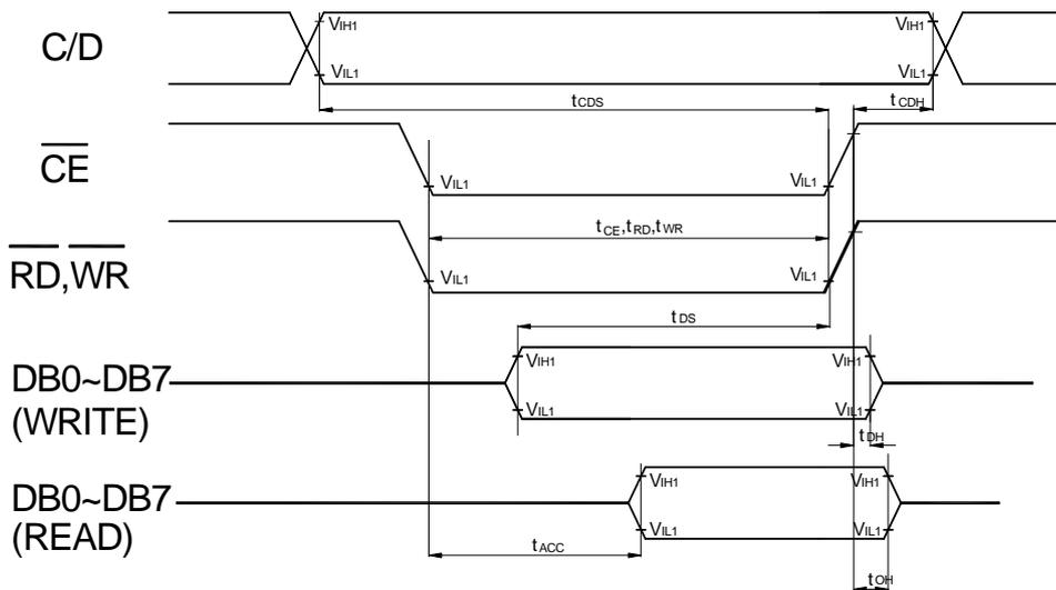
Fig. a Interface timing (data write/read)
