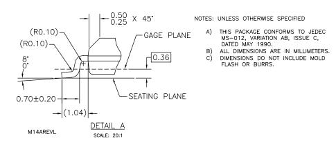
Figure 1. 14-Lead Small Outline Integrated Circuit (SOIC), JEDEC MS-012, 0.150" Narrow Package Number M14A
