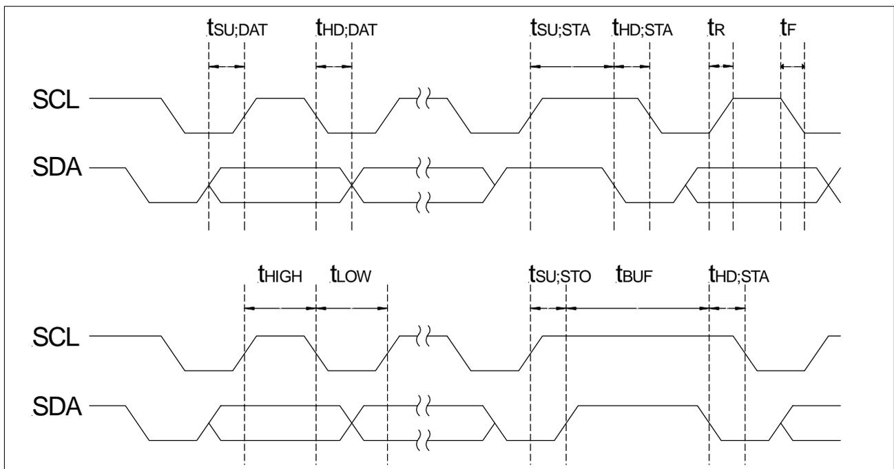
FIGURE II: Timing characteristics of the I<sup>2</sup>C interface
