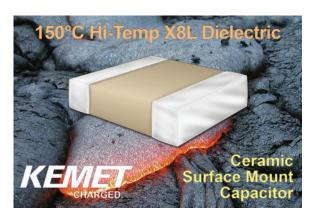
KEMET's X8L Dielectric offers an operating temperature range from -55°C to +150°C with capacitance shift limited to ±15% from -55°C to +125°C and +15, -40% from 125°C to 150°C. Product applications include harsh environments such as Down Hole (Oil Exploration), Automotive (Under Hood), Military and Aerospace.
