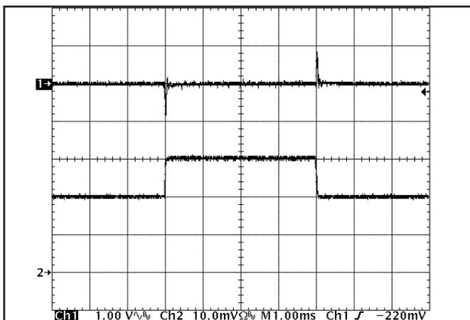
Figure 11: Output voltage response to step-change in load current (50%-75%-50% of  $I_{out(max)}$ ;  $dI/dt = 0.1A/\mu s$ ). Load cap: 15 $\mu F$ , 450 m $\Omega$  ESR tantalum and 1 $\mu F$  ceramic. Top trace:  $V_{out}$  (1V/div), Bottom trace:  $I_{out}$  (5A/div).
