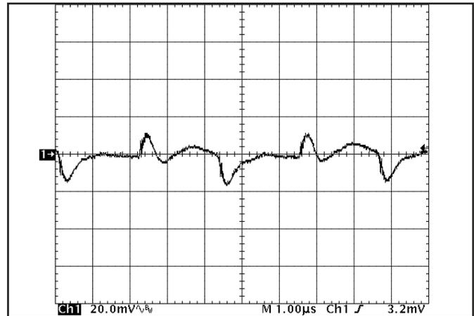
**Figure 16:** Output Voltage Ripple at nominal input voltage and rated load current ( $20\ \text{mV}/\text{div}$ ). Load capacitance:  $1\ \mu\text{F}$  ceramic capacitor and  $15\ \mu\text{F}$  tantalum capacitor. Bandwidth:  $20\ \text{MHz}$ . (See Figure 13)
