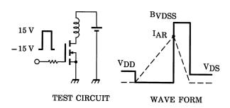
$$\begin{aligned} R_G &= 25~\Omega \\ V_{DD} &= 25~V,~L = 368~\mu H \end{aligned} \qquad E_{AS} &= \frac{1}{2} \cdot L \cdot I^2 \cdot \left( \frac{B_{VDSS}}{B_{VDSS} - V_{DD}} \right) \end{aligned}$$
