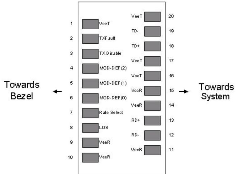
Figure 3 Transceiver pin descriptions
