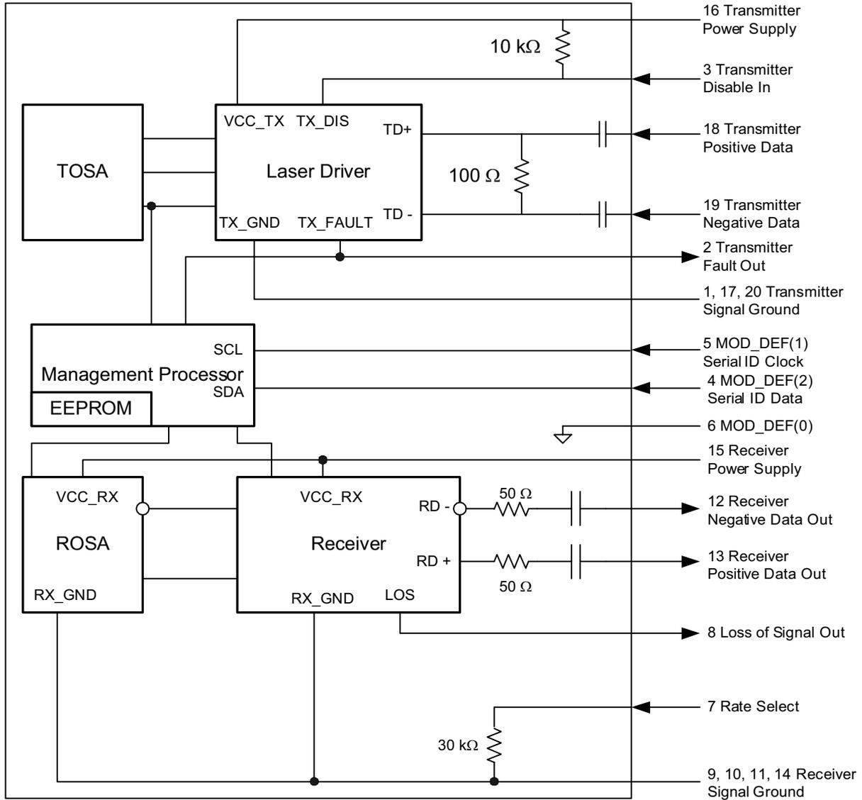
Figure 1 Block diagram
