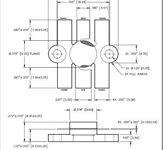
UNLESS OTHERWISE NOTED, TOLERANCES ARE INCHES  $\pm .005"$  [MILLIMETERS  $\pm 0.13$ mm]
