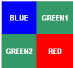
Figure 3. Color Filter Arrangement on the Pixels
