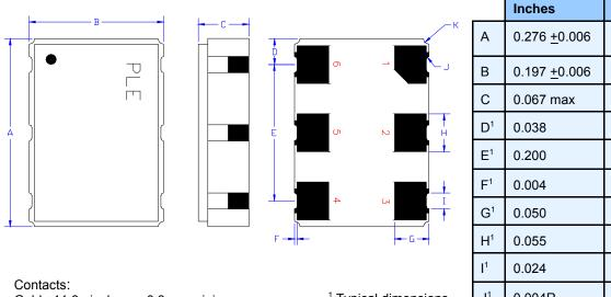
Gold 11.8 µinches 0.3 µm minimum over Nickel 50 to 350 µinches 1.27 to 8.89 µm
