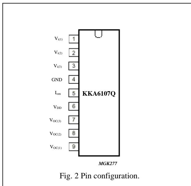
Fig. 2 Pin configuration.
