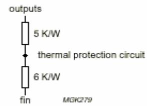
Fig.4 Equivalent thermal resistance network.
