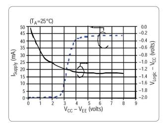
Figure 5. Typical supply current &  $\rm V_{Logic}$  vs. supply voltage
