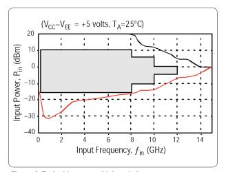
Figure 4. Typical input sensitivity window
