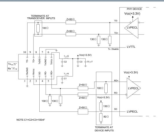
The split-loaded terminations for ECL signals need to be located at the input of devices receiving those ECL signals. The power supply filtering is required for good EMI performance. Use short tracks from the inductor L1/L2 to the module Rx Vcc. A GND plane under the module is required for good EMI and sensitivity performance.
