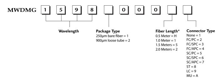
$<sup>^*</sup>$  The tolerance of fiber length is  $\pm$ 0.1m. 1 meter is standard. The lead-time for special fiber length will be longer.
