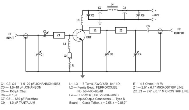
Figure 1. 400 MHz Power Gain Test Circuit
