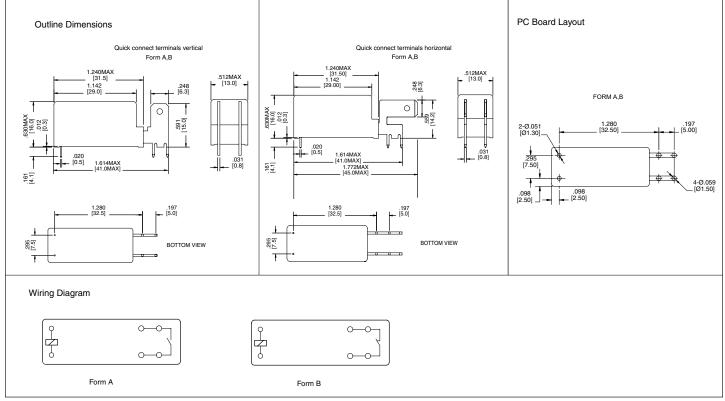
Dimensions in inch with millimeters in brackets below. Tolerance: ± .010"
