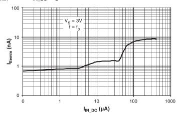
**Figure 6-2.**  $I_{Eemin}$  versus  $I_{IN\_DC}$ ,  $V_S = 5V$
