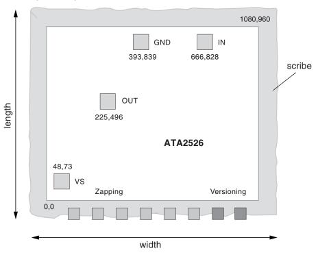
Note: Pad coordinates are given for lower left corner of the pad in  $\mu m$  from the origin 0,0
