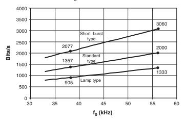
**Figure 6-6.** Data Transmission Rate,  $V_S = 5V$
