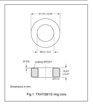
**Ring core data - Note** 1. Mechanical dimensions : OD  $\leq$  47.63, ID  $\geq$  27.89, H  $\leq$  16.13
