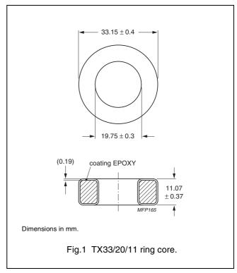
**Ring core data - Note** 1. Mechanical dimensions : OD  $\leq$  33.83, ID  $\geq$  19.3, H  $\leq$  11.61
