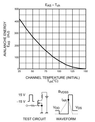
$\begin{array}{ll} R_G = 25 \; \Omega \\ V_{DD} = 90 \; V, \; L = 11.5 \; mH \end{array} \qquad E_{AS} = \frac{1}{2} \cdot L \cdot I^2 \cdot \left( \frac{BVDSS}{BVDSS} - V_{DD} \right)$
