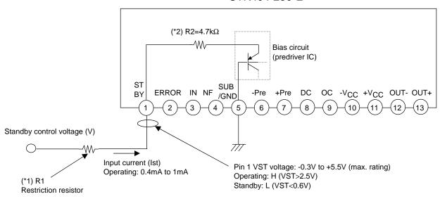
This pin has a function to release the latch when it is set to the ground level.
