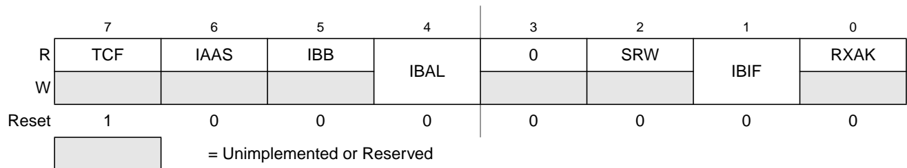
Figure 11-6. IIC Bus Status Register (IBSR)
