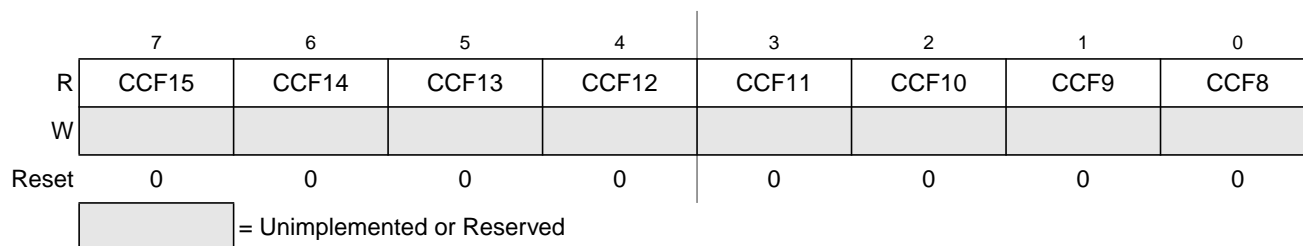
Figure 7-12. ATD Status Register 2 (ATDSTAT2)
