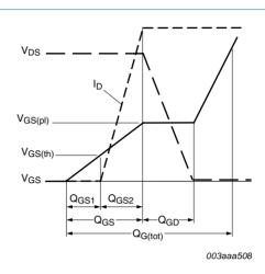
Fig 14. Gate charge waveform definitions
