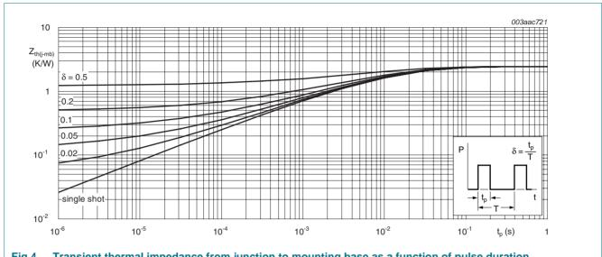
Transient thermal impedance from junction to mounting base as a function of pulse duration
