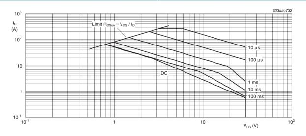
$T_{mb} = 25 \,^{\circ}C; I_{DM}$  is single pulse
