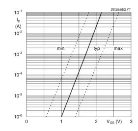
$T_j = 25 \,^{\circ}C; V_{DS} = 5 \, V$
