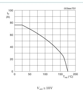
Continuous drain current as a function of
