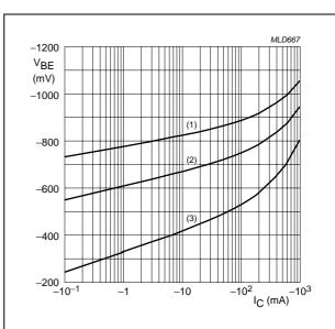
TR2 (PNP);  $V_{CE} = -2 \text{ V}$ .
