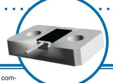
The PCS-P series split ground high power thin film terminator combines the improved heat dissipation of a double-sided flange and the split ground to give a power rating of up to 80W, while providing excellent high frequency characteristics from DC to 10GHz. Attaching the flange directly to a heat sink provides improved heat dissipation at a higher power rating. Typical applications include aerospace, wireless communication, satellites and RF power amplifiers
