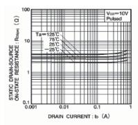
Fig.1 Static drain-source on-state resistance vs. drain current (I)
