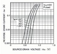
Fig.5 Reverse drain current vs. source-drain voltage (I)
