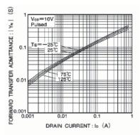
Fig. 7 Forward transfer admittance vs. drain current
