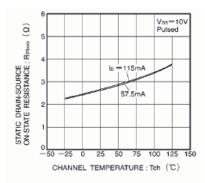
Fig. 4 Static drain-source on-state resistance vs. channel temperature
