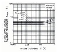
Fig. 2 Static drain-source on-state resistance vs. drain current (II)
