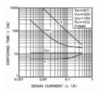
Fig. 9 Switching characteristics (See Figures 13 and 14 for the measurement circuit and resultant waveforms)
