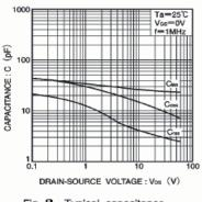
Fig. 8 Typical capacitance vs. drain-source voltage
