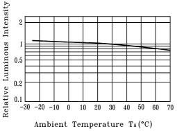
nbient Temperature Ta(°C) Fig.5 Luminous Intensity vs. Ambient Temperature
