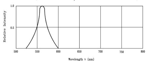
Fig.1 Relative Intensity vs. Wavelength
