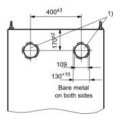
Connecting to shielding wall by flexible connector fittings (must be ordered separately)
