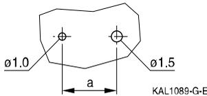
Suggestion for PCB hole diameter, wire ø1.0 mm
