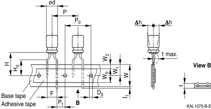
**Lead spacing 5.0 mm (from d × l = 10 × 12.5 mm to 12.5 × 30 mm)**
