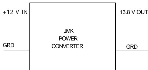
This small power supply is designed for use in automotive applications to power onboard computers, stereo equipment and other electronic hardware requiring a noise free and stable power input. This power supply is packaged in a small, sealed metal enclosure for maintenance free operation.
