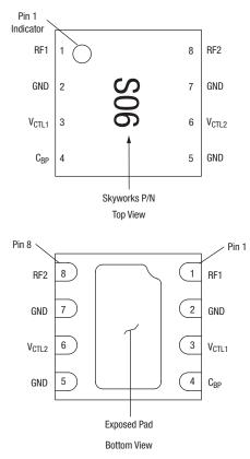
DC blocks are required on RF1 and RF2.  $C_{BLK}=560\ \text{pF}$  for 50 MHz operation.  $C_{BP}=560\ \text{pF}$  for 50 MHz operation.
